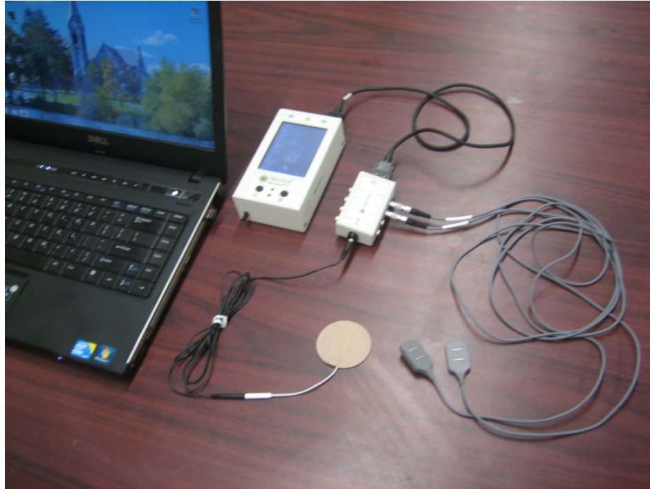
Figure 14. sEMG system suite used for collecting muscle activity data (DELSYS Myomonitor IV Wireless sEMG System).
